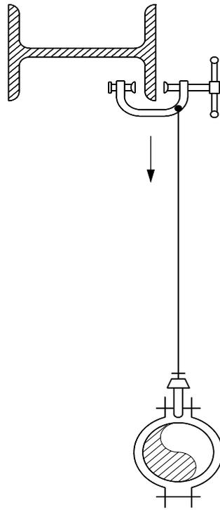
*Figure 3.4.5-1 C-Clamp Relies on Friction, May Slide*
