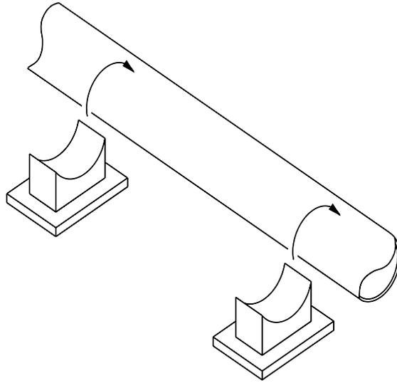
*Figure 3.4.3-1 Pipeline Lifts Off Shallow Saddles*
