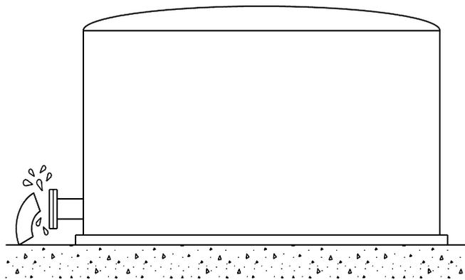
*Figure 3.4.1-2 Unanchored Flat Bottom tank Slides and Rocks*
