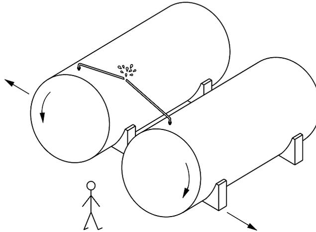
*Figure 3.4.1-1 Unanchored Tanks Slide and Twist on Saddles*
