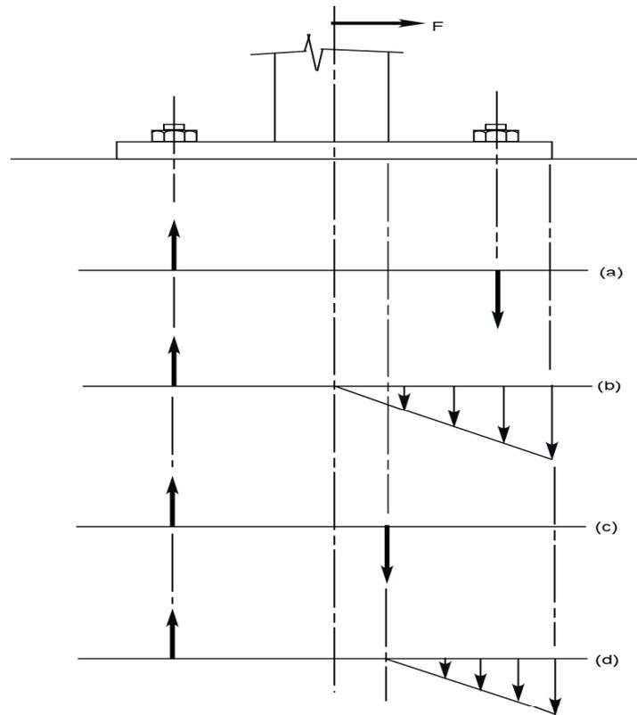
*Figure 8.3.3-1 Base Plate reaction to Overturning Moment*
