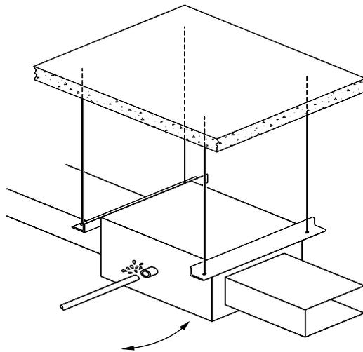
*Figure 3.4.4-2 HVAC Heater Sways and Ruptures Brazed Copper Tube*
