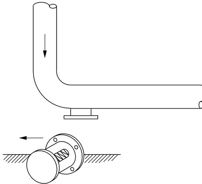
*Figure 3.4.5-4 Unanchored Spring Support Slides From Under Pipe*
