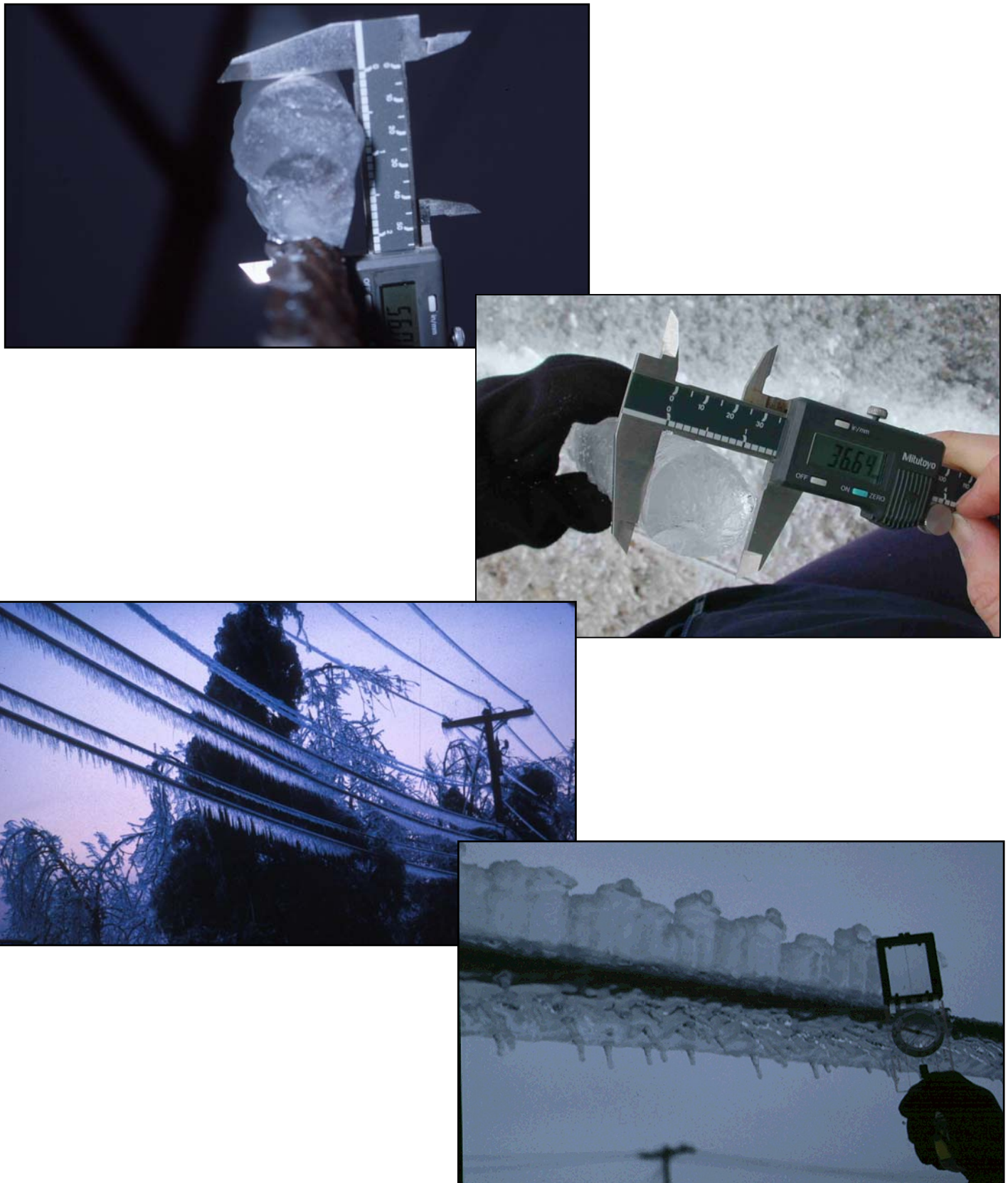
Figure 2.2-1 Some shapes of ice accreted from freezing rain on cylinders
