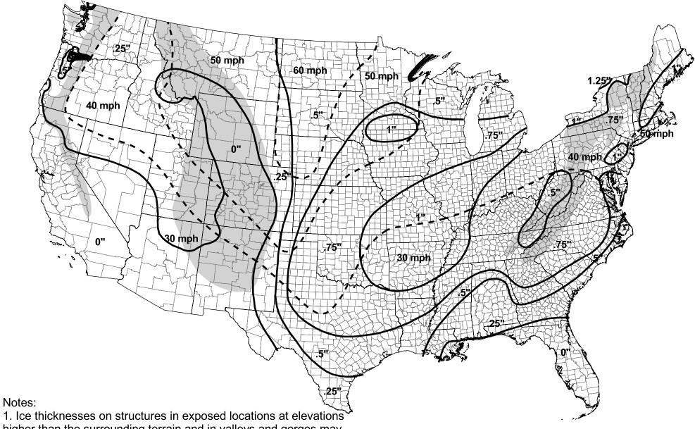
1. Ice thicknesses on structures in exposed locations at elevations higher than the surrounding terrain and in valleys and gorges may exceed the mapped values.
