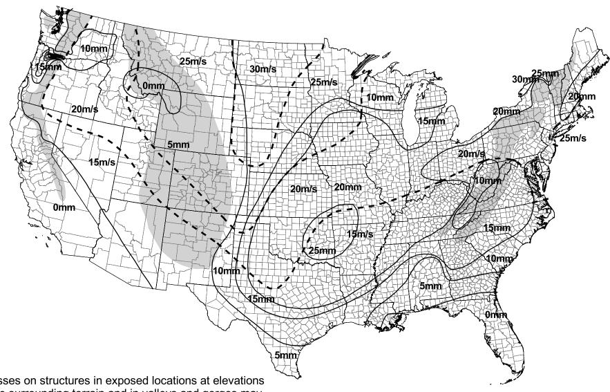
1. Ice thicknesses on structures in exposed locations at elevations higher than the surrounding terrain and in valleys and gorges may exceed the mapped values.
